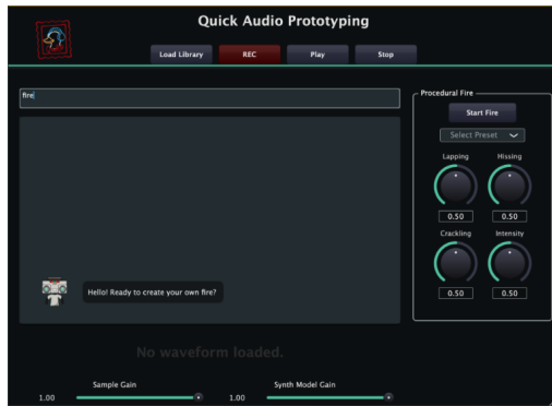
Figure 3: QuAP graphical user interface. The left panel displays the audio library search results, supporting both text-based and drag-and-drop similarity queries. The right panel exposes the procedural audio model controls, with the embedded assistant providing perceptually informed parameter recommendations.
