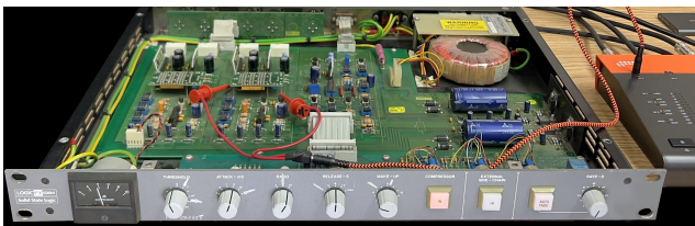
Figure 3: SSL Logic FX G384 bus compressor measured for dataset. The wire test leads are connected to the control input of the left audio VCA.
