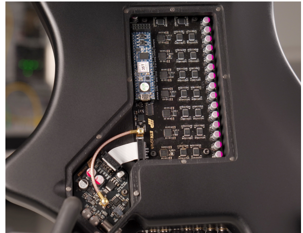
Figure 4: View of the back of the guitar, showing the control electronics (cover removed).
