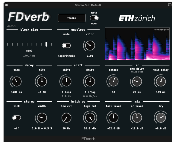
Figure 4: User interface of the FDverb plug-in with the real-time envelope visualization found at the top right.
