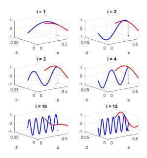
Figure 6: Modes of the coupled string-bridge system, which were normalized, and plotted orthogonal one to another for visualisation purposes. The letter *i* gives the mode index. The blue line represents the string, and red one the bridge, while the projection of the contact point on the z-axis is highlighted with a black dot. The physical parameters were the same listed in Figure 5, with  $\kappa_{\rm p} = 3.0619 \, {\rm N}^{1/2} \, {\rm m}.$
