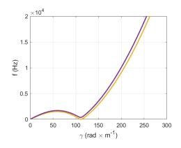
Figure 7: Plot of the dispersion relation of a thin spring. Physical parameters were chosen to be coherent with a possible yaybahar spring:  $R_{\rm c} = 9$  mm,  $r_{\rm c} = 1$  mm,  $\theta = 2^{\circ}$ ,  $L_{\rm c} = 40$  m,  $\kappa_{\rm c} = 9.9$ and  $\nu_c = 0.3$ . These values yield  $N_{\mathfrak{v}} = 2812$  within the hearing range.
