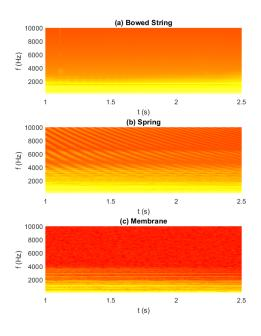
Figure 8: Spectrograms of the three subsystems outputs after the initial transient. Panel (a) displays the spectrogram of the extracted force  $F_p$ , panel (b) shows the spectrogram of the force signal  $F_c$ , and panel (c) represents the output signal  $\dot{w}_o$  at the output position  $(X_o, Y_o)$ .
