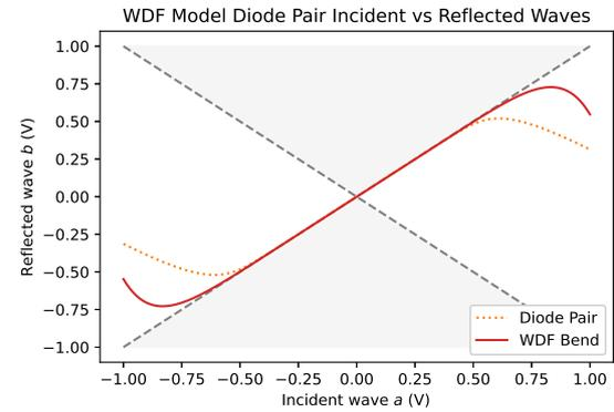
Figure 5: (orange) Explicit diode pair nonlinearity, (red) nonlinearity produced by (14) and (15). The white area represents the region of pseudopassivity, the grey area represents the region of pseudoactivity, and the dashed lines represent pseudolosslessness [26].
