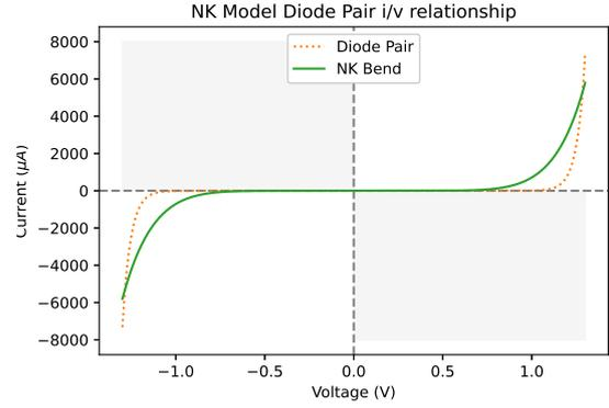
Figure 4: (orange) Explicit diode pair nonlinearity, (green) nonlinearity produced by (13) and (15). The white area represents the passive region while the grey area represents the active region.
