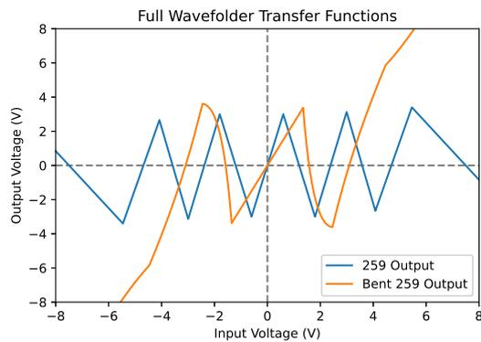
Figure 9: (blue) Transfer function of the entire Buchla 259 clipper. (orange) Transfer function of the entire Bent 259 clipper.
