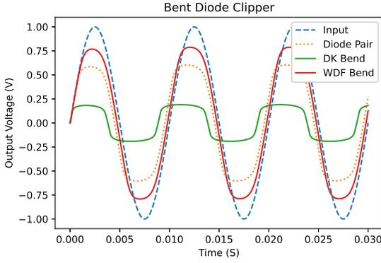
Figure 3: (blue) Sinusoidal input with frequency 100Hz, amplitude 1V, (orange) output of NK model using (11), (red) output of WDF model using (14) and (15), (green) output of NK model using (13) and (15).
