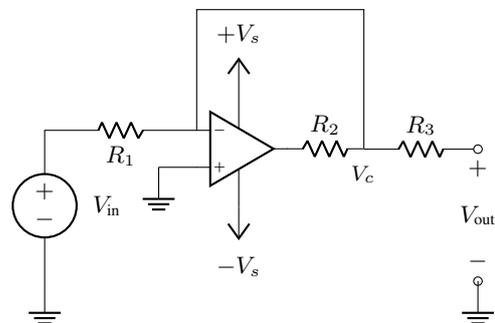
Figure 8: Circuit for a folding cell in the Buchla 259
