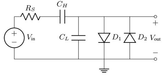
Figure 1: Two-capacitor diode clipper circuit.
