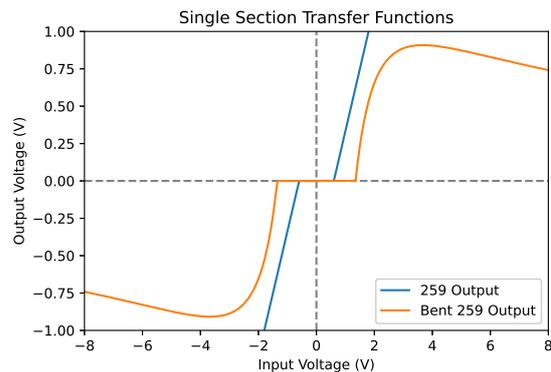
Figure 7: Center clipping wavefolder sections from both the Buchla 259 (blue), produced by (18), and the Bent 259 (orange), produced by (23).
