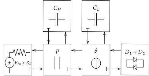
Figure 2: Two-capacitor diode clipper WDF tree.
