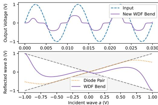
Figure 6: Top: (blue) Sinusoidal input with frequency 100Hz, amplitude 1V, (purple) output of (16). Bottom: (purple) a-b characteristic of (16), (orange) diode a-b characteristic for reference.
