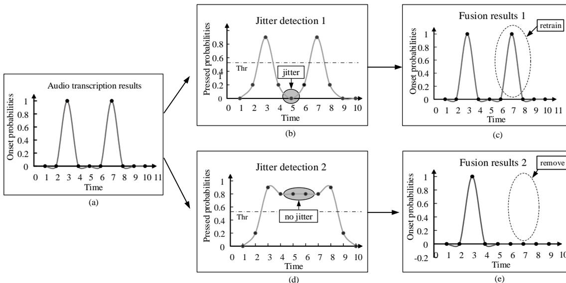
Figure 7: Jitter is used to eliminate successive errors.
