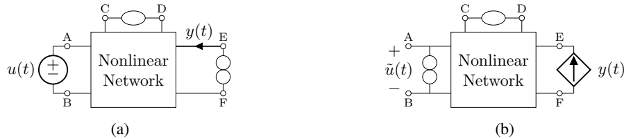
Figure 5: (a) shows a nonlinear non-autonomous system with at least one nullor (the master). The input signal u(t) is a voltage source, while the output signal y(t) is the current through the norator. (b) shows the inverse system (the slave) of the one in (a). Letters A, B, C, D, E and F indicate the same nodes of the nonlinear network both in (a) and (b).
