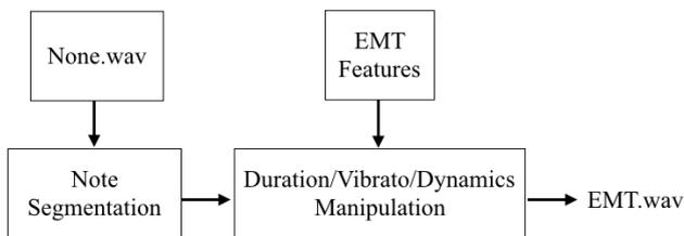
Figure 1: Flowchart of the EMT synthesis system.
