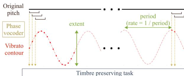
Figure 2: Illustration of adding vibrato to a non-expressive note. The note is divided into a sequence of fragments whose pitches will be individually shifted by means of the phase vocoder. The timbre preservation is applied to each fragment. The vibrato contour is sampled at sixteen times per cycle to avoid artifacts.
