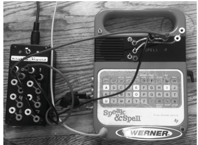
Figure 1: Circuit-bent Speak & Spell with MIDI control, Kurt James Werner, 2007
