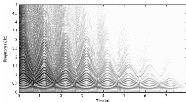
Figure 5: Control rate modulation of dispersion amount.  $B$  is swept between 0 and 0.01, using a sinusoidal LFO with 1 Hz rate as the modulating source.
