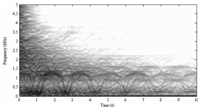
Figure 6: Audio rate modulation of the dispersion allpass. White noise excitation, 65.4 Hz fundamental frequency, 64.4 Hz sinusoidal modulation, and maximum  $B$  deviation of 0.005.
