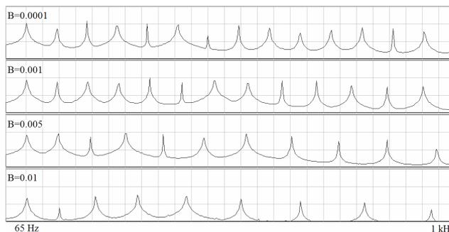
Figure 4: The lower part of displacement spectrum (20..1000 Hz) with various values of dispersion amount  $B$ . Linear frequency scale,  $f_0 = 65.4$  Hz.
