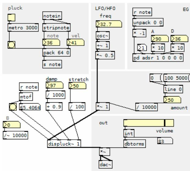
Figure 2: PD implementation. The string and dispersion model is within the *displuck~* external, also implemented in this work.
