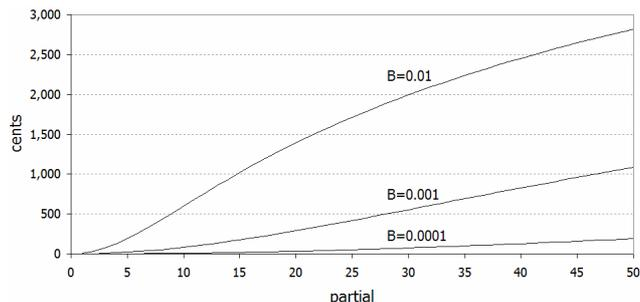
Figure 1: The effect of dispersion to partial detuning, according to stretching equation (1).
