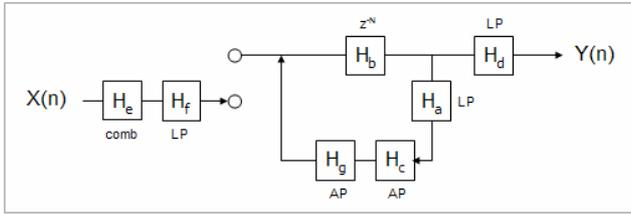
Figure 3: Extended Karplus-Strong algorithm (adopted from [8]). LP denotes low pass and AP allpass filter.  $X(n)$  is the excitation signal, while  $Y(n)$  is the output.  $H_g$  is the dispersion allpass.
