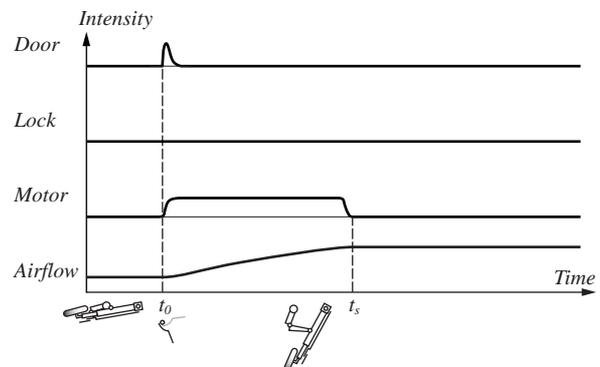
Figure 6: Example extension of landing gear gets stuck.
