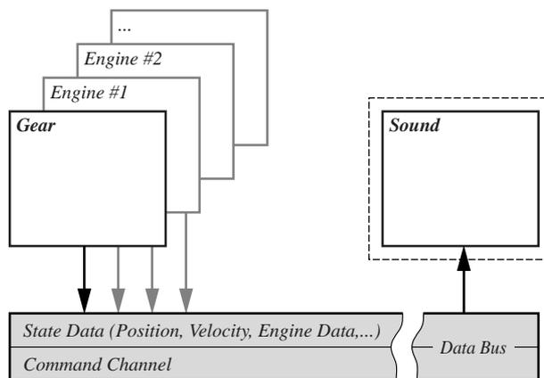
Figure 8: Interaction between Modules and Sound Rendering Engine.
