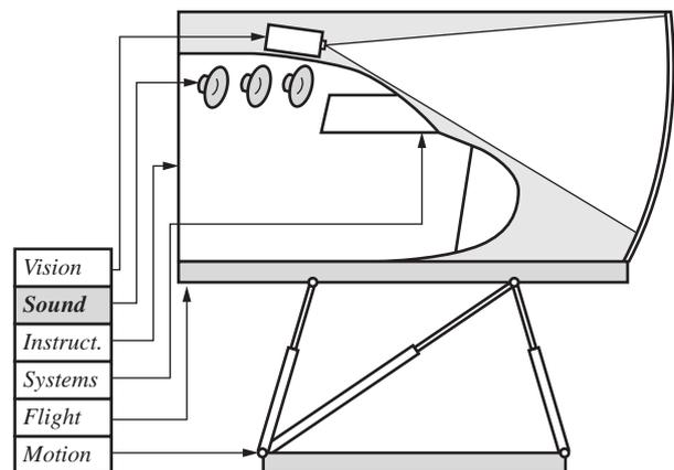
Figure 1: System components of a flight simulator.
