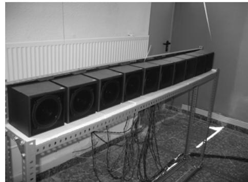
Figure 11: Loudspeaker array
