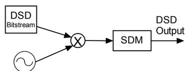
Figure 4: Modulation of a DSD bitstream.
