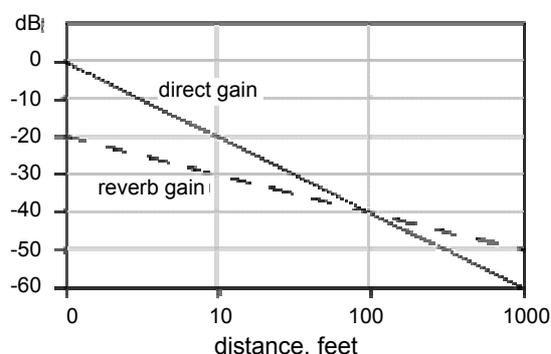
Figure 1: An example of direct to reverb energy ratio [3].
