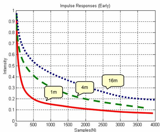
Figure 5: Shapes of early reflections with distances.
