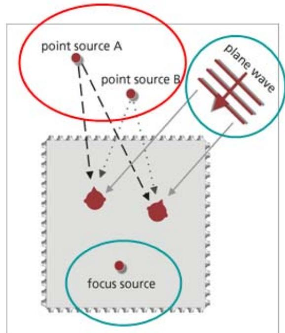
Figure 2: Reproduction of point source, focused sources and plane waves with WFS
