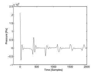
Figure 7: Impulse response of a brass instrument simulated at a sampling rate of 44100 kHz. The parameters of the model are adjusted to fit the measures of a trumpet.
