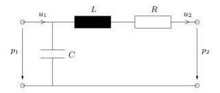
Figure 4: Analogous acoustic network for a brass mouthpiece.
