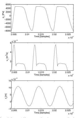
Figure 8: State variables  $p_1$ ,  $u_1$  and  $x_1$  of a trumpet tone. Simulation was carried out at a sampling rate of 44100 kHz.
