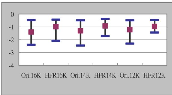
Figure 12: The ODG range of the mp3 and H.F.R audio with different cut-off frequencies under 128k bit rate.
