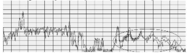
Figure 5: Spectrum of the compressed audio signal with bandwidth extension.
