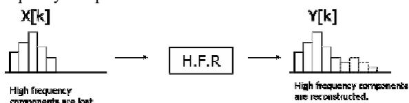
Figure 1: Block diagram of audio bandwidth extension
