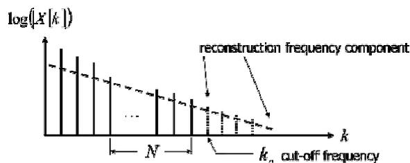
Figure 2: Linear extrapolation on the magnitude with logarithm scale
