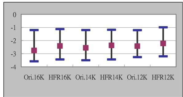
Figure 16: The ODG range of the mp3 and H.F.R audio with different cut-off frequencies under 96k bit rate.
