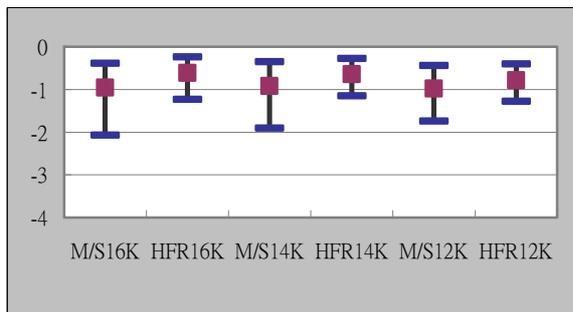
Figure 14: The ODG range of the mp3 with M/S coding and H.F.R audio with different cut-off frequencies under 128k bit rate.
