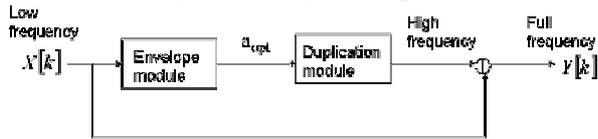
Figure 6: A block diagram of audio bandwidth extension.
