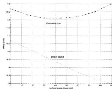
Figure 9: Delay of direct sound ( $\rho_1$ ) and first reflection ( $\rho_2$ ) measured in the auditorium excited by the experimental device shown in figure 8.
