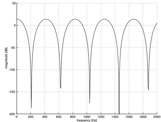
Figure 5: Frequency response of the two-path system for a delay difference of 2.4 ms and  $\alpha = 1$ .
