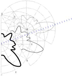
Figure 6: Directivity pattern at the frequency  $f = 2,352\text{Hz}$  plotted for three clarinet angles with respect to the mouthpiece.
