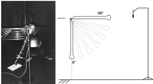
Figure 8: Room response measurements with excitation provided by a loudspeaker connected to a clarinet tube.
