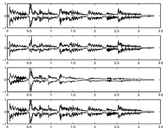
Figure 4: Sound source separation in a piece for two guitars (Top to bottom): A: Recorded signal, left channel. B: Separated signal, rythm part. C: Separated signal, solo part. D: Recorded signal, right channel.
