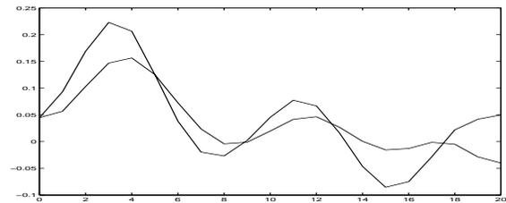
Figure 2: Magnitude of coefficients in demixing matrices as a function of delay. Upper curve: source 1 to sensor 2. Lower curve: source 2 to sensor 1.
