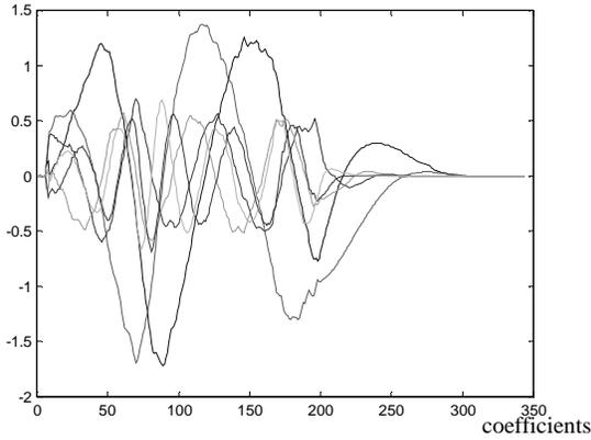
Figure 4. HB scale analysis coefficients of a violin sound at 294 Hz, 3 harmonics, i.e., 6 analysis channels.
