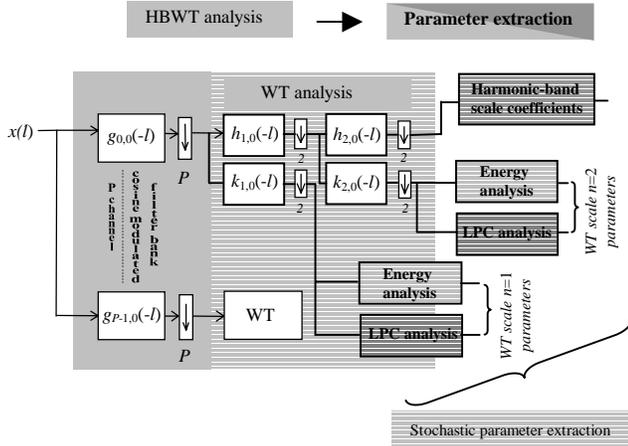
Figure 2. Harmonic-Band Wavelet (HBWT) analysis scheme and resynthesis parameter estimation. The  $g_{p,0}(l)$  represent the impulse responses of the filters implementing a MDCT. The  $h_{n,0}(l)$  and  $k_{n,0}(l)$  represent the impulse responses of pairs of QMF filters implementing a wavelet transform.
