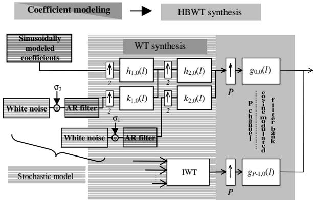
Figure 3 Harmonic-Band Wavelet (HBWT) resynthesis scheme
