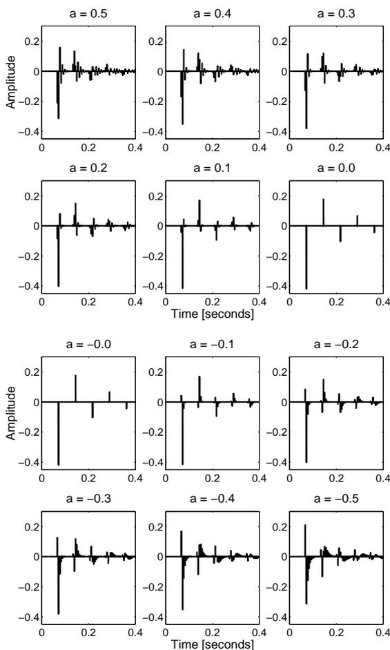
Figure 4: Impulse responses of one channel at different  $a_i$  values.
