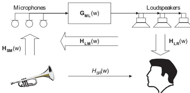
Figure 1: The transfer functions present in all RESs, after [1].
