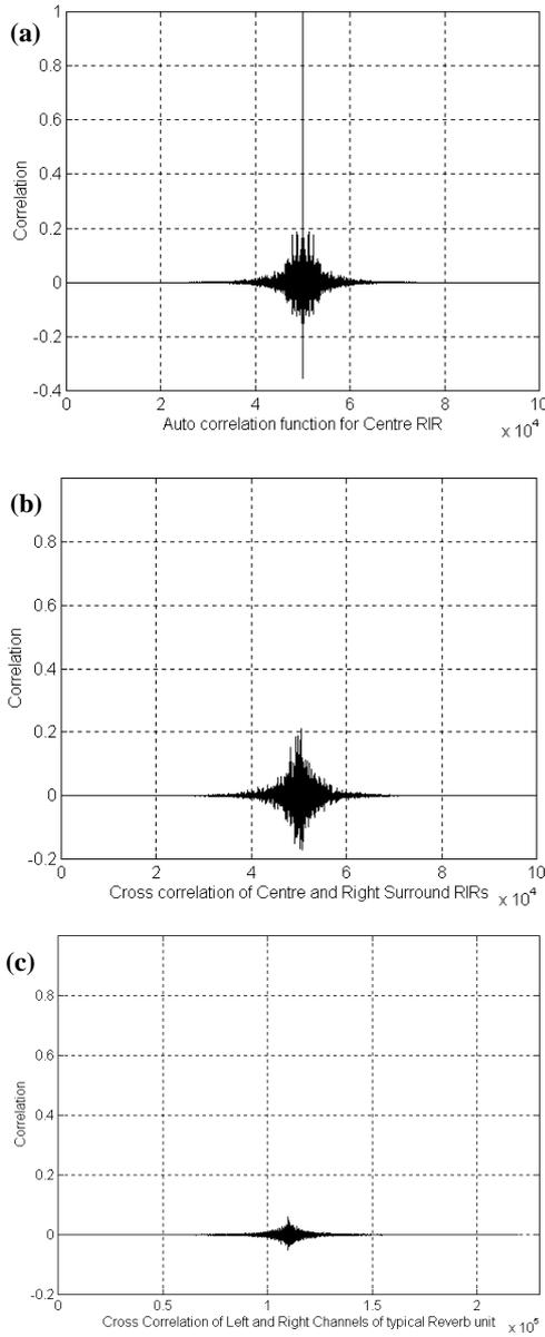
Figure 3: Cross-correlation functions for surround output RIRs. (a) The normalised autocorrelation function for the Centre RIR; (b) the normalised cross-correlation function for the Centre and Right Surround RIRs; and (c) for comparison the normalised cross-correlation function for the left and right channels of a typical filter based reverberator.
