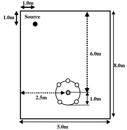
Figure 2: Plan view of the modelled room showing positions of input sound source and 5.1 RIR measurement points based around a central output position.
