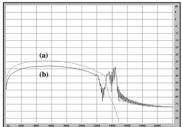
Figure 5: Frequency response of incident and reflected waves at a boundary on the triangular mesh with  $r = 1.0$ . (a) Incident wave; (b) Reflected wave.
