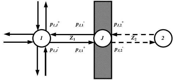
Figure 4: Termination of a waveguide mesh due to a boundary resulting in a reflection.
