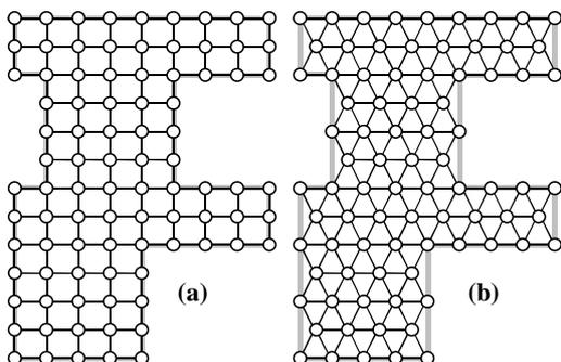
Figure 2. A simple 2-D enclosed space and the resultant mesh structures used. (a) rectilinear mesh topology; (b) triangular mesh topology.
