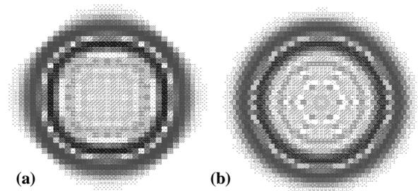
Figure 4. Wavefronts on, (a) rectilinear mesh, and (b) triangular mesh, 14 time steps after an applied Gaussian impulse.
