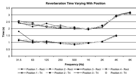
Figure 6. Reverberation Time Measurements varying with output point position in the modelled room, for both the triangular mesh (upper set of measurements) and the rectilinear mesh (lower set of measurements).
