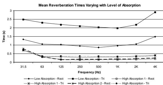
Figure 7. Spatially Averaged Reverberation Time Measurements, varying with level of absorption in the modelled room.
