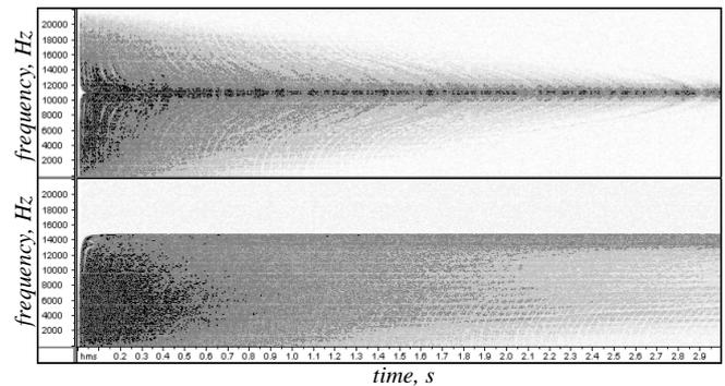
Figure 5. Time varying spectral analysis of RIR from a single output point for, (top) rectilinear mesh, and (bottom) triangular mesh.
