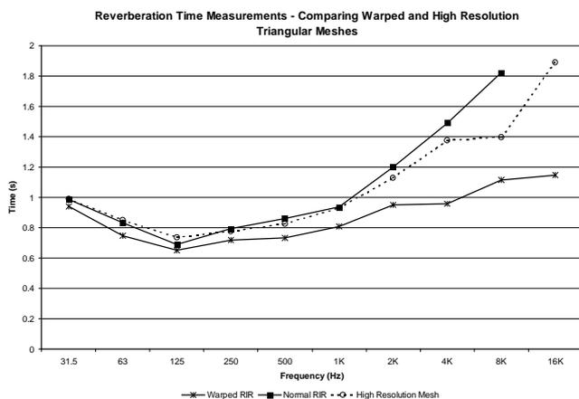
Figure 8. Reverberation Time measurements for the triangular, high-resolution triangular, and warped triangular mesh structures.
