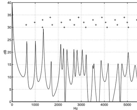
Figure 2: Frequency response of the parallel of dispersive comb filters designed for radius 0.188.  $+$ : resonance positions of the ideal sphere up to Bessel series of order 4.
