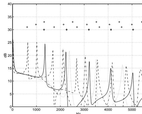
Figure 3: Superimposition of the responses of the dispersive comb filters designed for radius 0.188. Solid line: Bessel order 0. Dashed line: Bessel order 1. Dash-dotted line: Bessel order 2. Dotted line: Bessel order 3.
