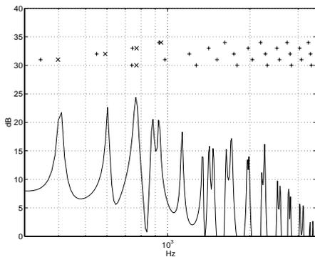
Figure 5: Frequency response of the FDN model of the plastic ball. +: resonance positions of the ideal sphere. x: measured resonance positions.
