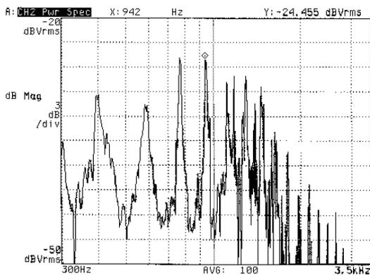
Figure 4: Measured frequency response of the plastic ball.
