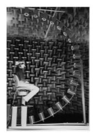
The tracking control, to avoid head movements during the measurements, is made with a laser beam positioned and fixed on the head of the subject. The laser beam has to aim at a target for any azimuth position.
