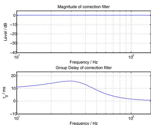
Figure 6: Magnitude and group delay response of the correction filter before time-reversal
