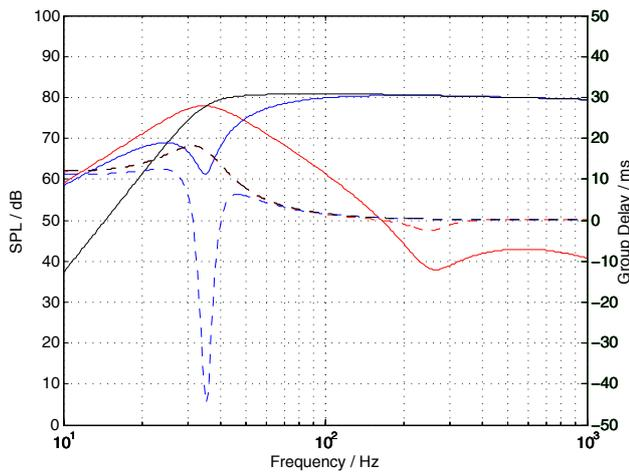
Figure 1: Splice simulation of vented box showing magnitude (—) and group delay (- -) responses of the driver (blue), the port (red) and the combined output (black).
