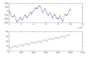
Figure 1: Unwrapped and de-trended phase for a concert A recorded from a violin (above) and a windowed sample of the signal (below) showing a series of replica phaselets associated with the primary resonance characteristics of the instrument.
