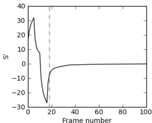
Figure 2: The first derivative of spectral flux  $S$  plotted against time. The beginning of the resonance as a dashed vertical line.
