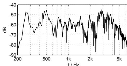
Figure 2: *Magnitude frequency response ('resonance profile') of a violin body.*
