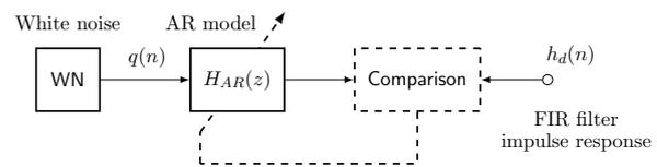
Figure 3: Autoregressive model which forms a white noise input signal to have similar spectral properties as the FIR filter used for resonance modifications.
