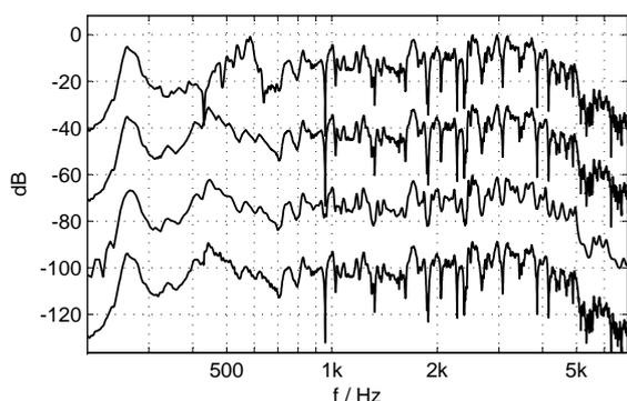
Figure 8: Example of modification of the first violin corpus resonances. From top down, separated with 30 dB offset: Original violin resonance profile, desired new resonance profile, spectrum of the complete AR model, and spectrum of the modified impulse response (method b), see also description in the text and Fig. 7). In both cases, the AR order is  $p = 250$ .
