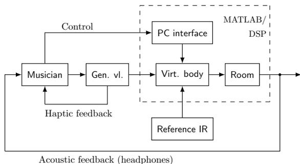
Figure 11: Main components of the violin platform: the virtual body filters the string signals of a silent generator violin (Gen. vl.). Impulse responses of real violins (Reference IR) are used as starting point for further resonance modifications. The ‘Room’ block represents a standard reverberation effect.
