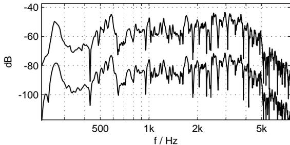
Figure 6: Top: Spectrum of an AR model (order  $p = 1500$ ) without frequency warping. Bottom ( $-30$  dB): Spectrum of an AR model which is computed with frequency warping (order  $p = 250$ ).
