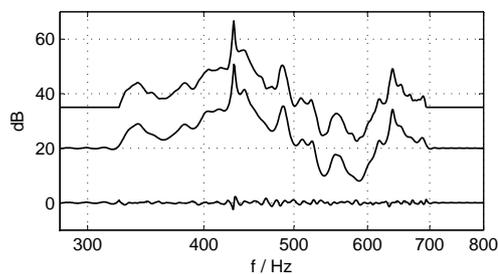
Figure 10: From top down: Example difference spectrum (+35 dB offset, description in the text), spectrum of the modification filter (AR order  $p = 250$ , +20 dB offset), and the corresponding frequency-dependent error.
