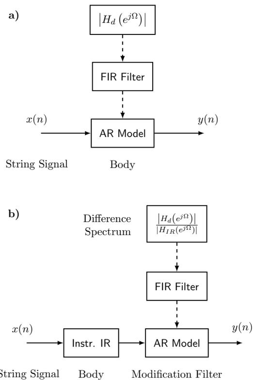
Figure 7: The two body modeling options (see description in the text): a) The virtual instrument body is completely realized by an AR model which approximates the desired resonance profile  $|H_d(e^{j\Omega})|$ . b) The difference spectrum between the desired resonance profile and the original resonance profile  $|H_{IR}(e^{j\Omega})|$  is the magnitude frequency response of a modification filter.
