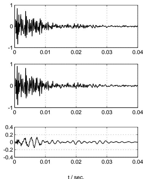
Figure 9: Original violin impulse response (top) in comparison to the modified impulse response (middle, see example in the text). Bottom: difference plot.
