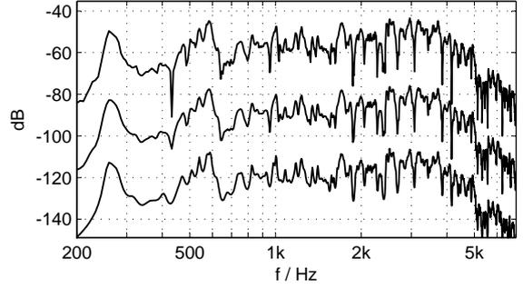
Figure 4: From top down, separated with 30 dB offset: Original violin resonance profile, magnitude spectrum of the high-order FIR filter (order  $N_F = 8000$ ), and magnitude spectrum of the corresponding high-order AR model (order  $p = 1500$ ).
