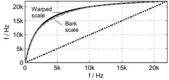
Figure 5: Frequency scales: linear (dotted), Bark (Zwicker & Fastl, gray, dashed), and warped ( $\lambda = 0.75$ , black, solid).
