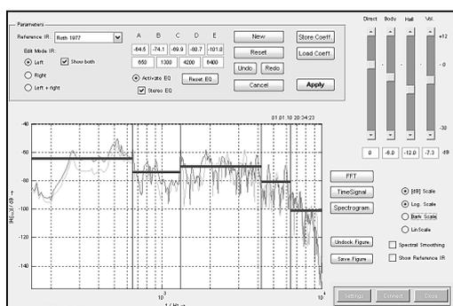
Figure 12: MATLAB GUI with magnitude frequency response plot for defining modifications of resonance profiles. The horizontal lines in the spectrum plot represent an additional audio equalizer function [15].
