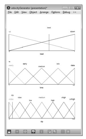
Figure 2: Membership functions used to fuzzify the inputs **beat** (top) and **time** (middle) in Max5. The output of the fuzzy controller is the amount of velocity attenuation, **dip** (bottom).
