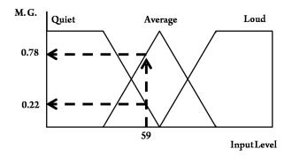
Figure 1: Determination of fuzzy membership grades (M.G.) of an input of 59 using membership functions.
