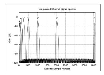
Figure 5: Channel-frequency-response overlay for a complexsignal octave filter bank, designed using a length 127 Dolph-Chebyshev window (80 dB stopband attenuation) and length 256 FFT.
