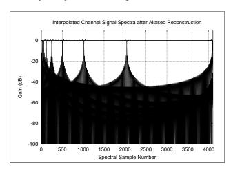
Figure 6: Same as Fig. 5 obtained by critically downsampling each channel signal, zero-padding, and performing an FFT. All the observable stopband error happens to cancel out in the filter-bank sum because the input signal is an impulse, in which case the reconstruction remains exact.
