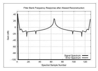
Figure 8: Signal spectrum (an impulse, since the time signal is a step) and error spectrum for the case of Fig. 7. Note the large error near half the sampling rate.
