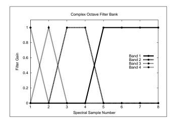
Figure 2: Simple octave filter bank for complex signals.
