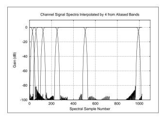
Figure 10: Same example as in Fig. 9 but looking at the effects of aliasing to to channel-signal downsampling. Compare to Fig. 6.
