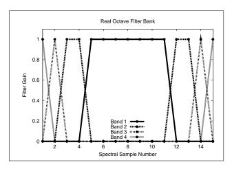
Figure 3: Simple octave filter bank for real signals.
