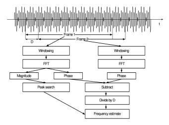
Figure 1: Block diagram of precise frequency estimates
