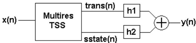
Figure 4. *Percussive post-processing algorithm. Once the signal has been split using the multiresolution TSS separation algorithm, resulting signals are filtered separately to produce hard/soft percussive attacks.*
