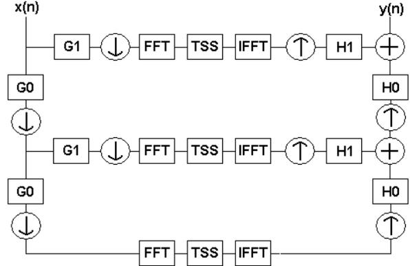
Figure 1. Octave spaced filter bank implementation. Only two subband levels are shown here, whereas six bands are used in the actual implementation.
