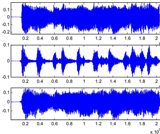
Figure 2. Separation of a strummed guitar signal (top) into transient/noise (center) and steady state (bottom) parts.
