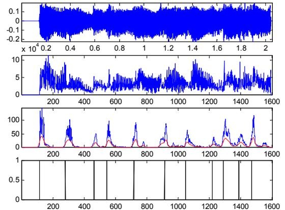
Figure 3. Comparison between standard HFC content (upper middle) and TSS separated transient only HFC content (lower middle) of strummed guitar signal (top) yielding near-perfect onset detection (bottom).
