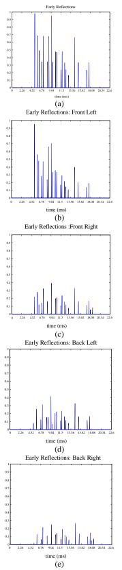
Figure 7. Early reflections for a virtual room before (a) and after (b)-(e) the sound panning process (see text).
