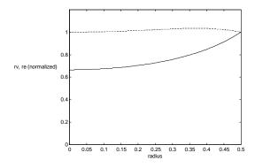
Figure 4. Evolution of the amplitude of normalized velocity vector (solid) and normalized energy vector (dotted) with the radius.
