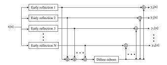
Figure 8. Directional reverberator block diagram
